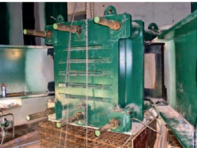
Seismically stable Abutment with 6 DYWIDAG Bars
