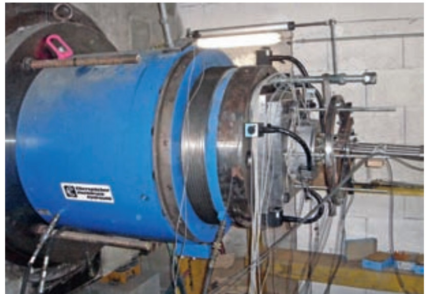
Hydraulic Cylinder with mounted Anchorage and Measuring Equipment
