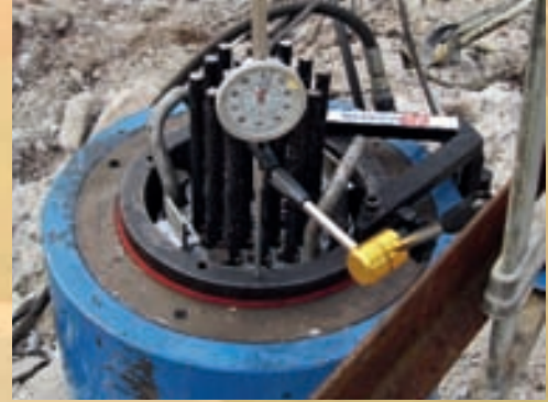
Performance tests at permanent SUSPA Strand Anchors at 3.320kN
